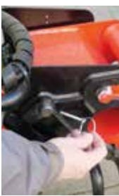
Insert the mechanical pin and the safety lock pin
