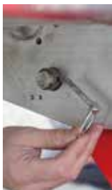
Remove the mechanical pin (type B winch)
