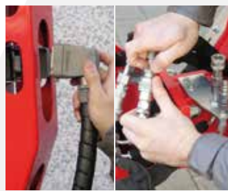
Connect the electrical connector and attach the hydraulic hoses
