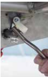
Remove the mechanical pin (type B winch)
