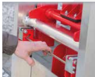
Release the mechanical lever (Type A winch)
