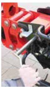
Insert the mechanical pin and the safety lock pin
