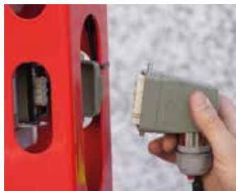
Disconnect the electrical connector
