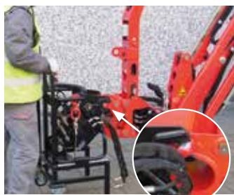
Attach the winch to the appropriate support pins
